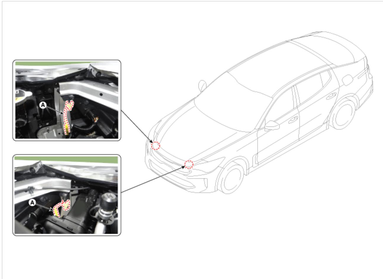
3. Remove the front impact sensor mounting bolt (A).
